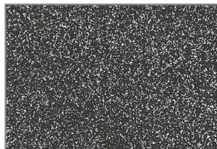
Powder Metallurgy steel has small, evenly distributed carbides
