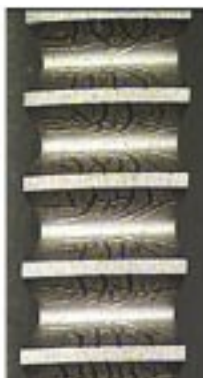
Tap after thread grinding (left) and after hot-hydrochloric-acid etching (right). The region exhibiting oxidation burn is on the unground surface. However, this is not a region with genuine, severe thermal damage. The thread-ground surface suffered the highest residual stress. However, this surface is clean – i.e., shows no oxidation burn – due to ‘cleaning up’ of the thin oxide layer.
