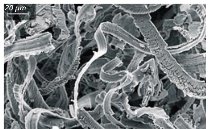
Above: Grinding swarf. Grinding is a chip-formation process (grinding of M9V with WA46HV wheel, 1000X).
