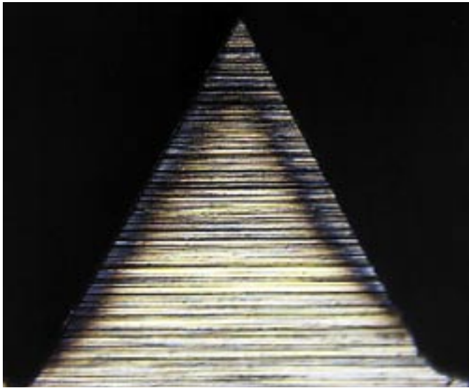
Oxidation burn on a tap. The surface is discoloured due to heat conduction from the thread-grinding operation. It does not indicate whether other types of thermal damage are present.
