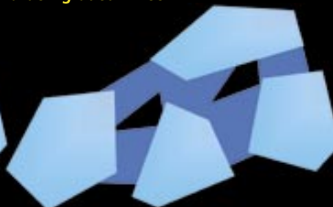
A softer-graded wheel and a harder-graded wheel. Harder-graded vitrified-bonded wheels have more bond material.
