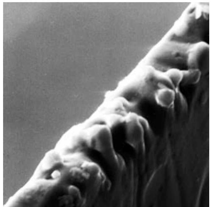
The edge of a knife made of ASP 2053. The carbides give the knife its wear resistance, but also make it more difficult to grind.
