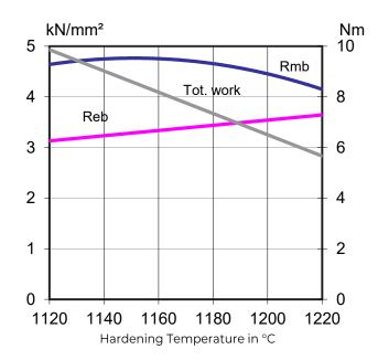
Tempering 3 x 1 hour at  $560^{\circ}$ C Dimension of test piece Ø 4.7 mm
