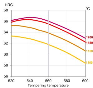
Hardness after hardening, quenching and tempering 2x1 hour
