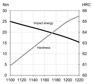
Hardening temperature in °C Tempering 2 x 1 hour at 560° C Unnotched test piece 7 x 10 x 55 mm
