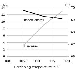
Original dimension  $\emptyset$  101 mm Tempering 3 x 1 hour at 560° C Unnotched test piece 7 x 10 x 55 mm
