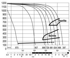
Continuous cooling transformation curve Hardening Temperature 1150°C
