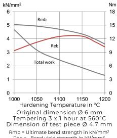
Rmb = Ultimate bend strength in kN/mm² Reb = Bend yield strength in kN/mm² Tot. work = Total work in Nm
