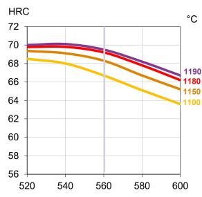
Hardening Temperature °C Hardness after hardening, quenching and tempering 3x1 hour
