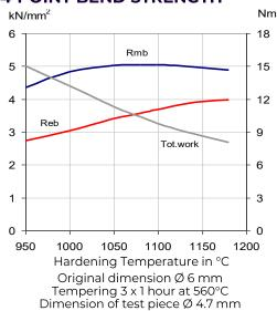
Rmb = Ultimate bend strength in kN/mm² Reb = Bend yield strength in kN/mm² Tot. work = Total work in Nm
