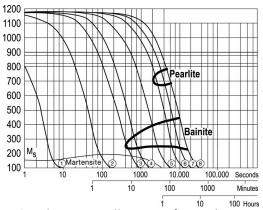
Continuous cooling transformation curve Hardening Temperature 1180°C
