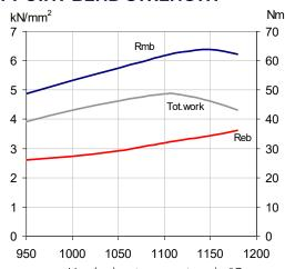
Hardening temperature in  $^{\circ}\text{C}$ Original dimension Ø 6 mm Tempering 3 x 1 hour at 560°C Dimensions of test piece Ø 4.7 mm
