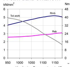
Hardening Temperature in °C Original dimension Ø 7.5 mm Tempering 3 x 1 hour at 560°C Dimension of test piece Ø 4.7 mm
