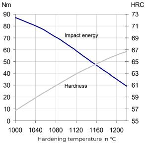
Original dimension Ø14 mm Tempering 3x1 hour at 560° C Unnotched test piece 7x10x55 mm
