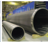
Suction Roll Shell for Paper Machine
